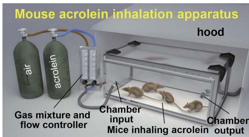
Fig. 1. The inhalation setup. Two gas cylinders, 350 ppm acrolein:air mixture and compressed air, were connected to the chamber inlet. Concentration was controlled by adjusting flow using two flowmeters. A chamber housed the mice and was placed in a chemical ventilation hood. Expired air from the chamber flowed through an outlet connected to a charcoal adsorption filter.
