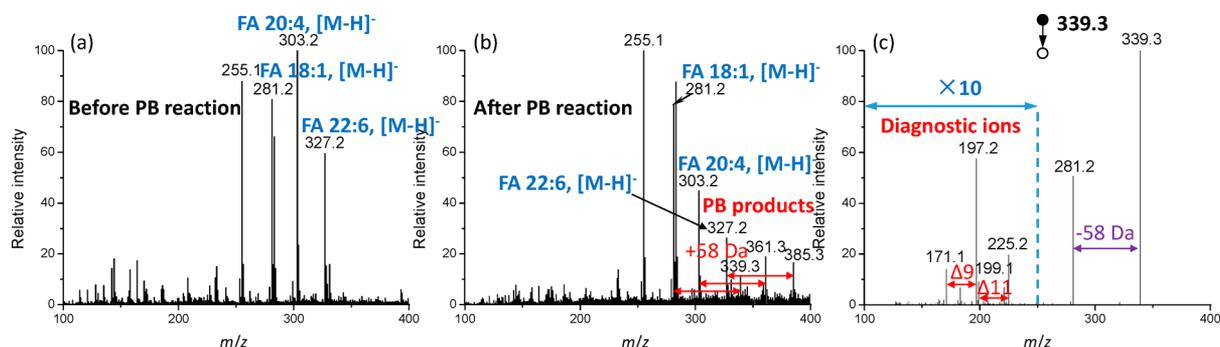
**Figure 4.** Mass spectrum of rat brain section by LMJ-SSP/PB reaction/ESI in negative ion mode before (a) and after (b) PB reaction. (c) MS/MS spectrum of the PB reaction products at  $m/z$  339.3.
