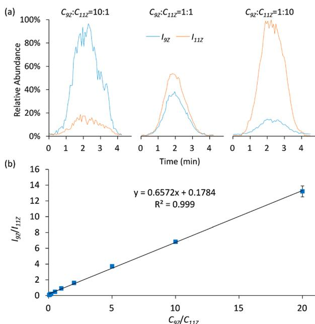
**Figure 5.** (a) Extracted ion chromatogram for FA 18:1 (9Z) and FA 18:1 (11Z) obtained from a standard mixture in different proportions. (b) Linear relationship established between diagnostic ion ratio and molar ratio of the two FA 18:1 C=C location isomers.
