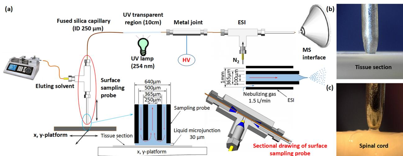
**Figure 1.** (a) Schematic of the experimental setup for profiling unsaturated lipid isomers. (b) Direct sampling of tissue section. (c) Direct sampling of mouse spinal cord.
