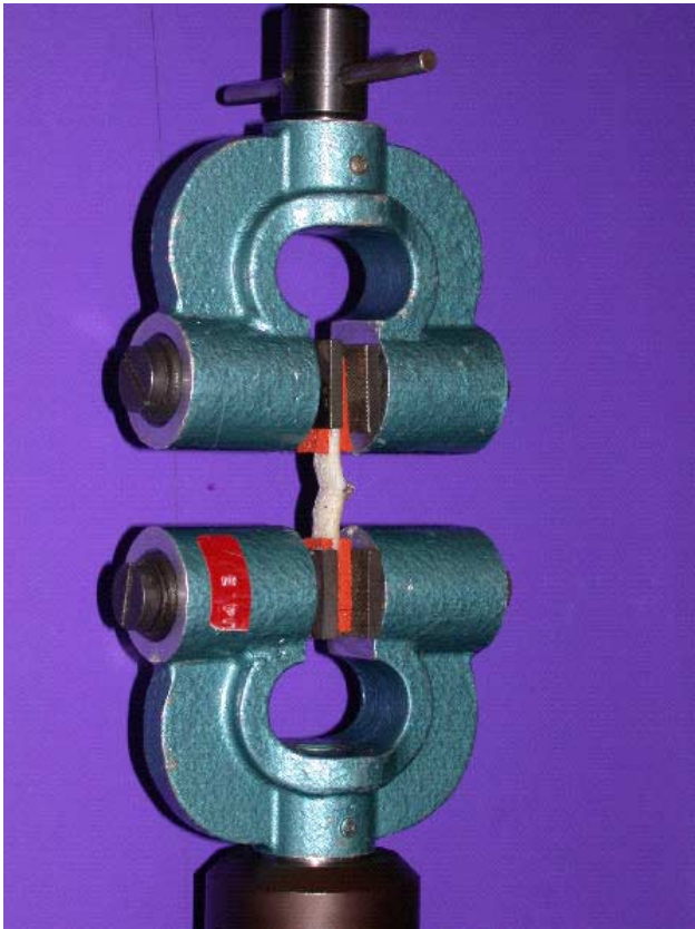
Fig. 2. Test fixture holding a cured skin specimen readied for testing to failure.
